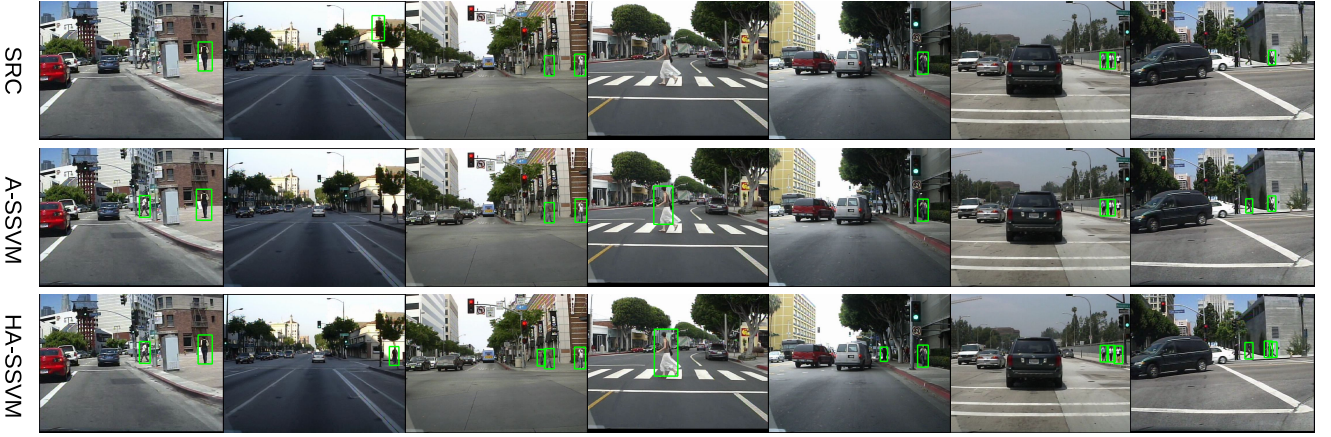
Fig. 7 Pedestrian detection on Caltech dataset for SRC, A-SSVM and HA-SSVM based models. The results are drawn at FPPI = 0.1.
