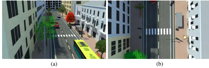
Fig. 2 Example of inverse perspective mapping from (a) oblique view; into (b) top view.
