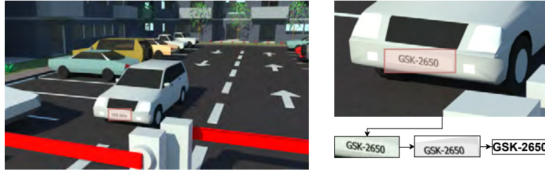
Fig. 4 Illustration of vehicle license plate recognition process for access control.
