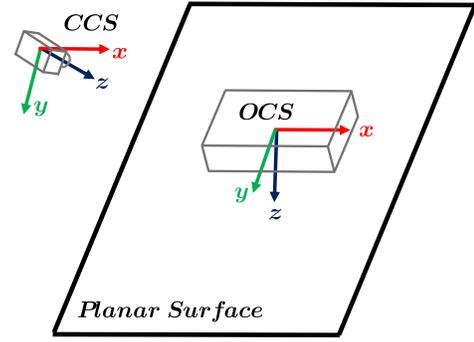
Fig. 1. Representation of the Camera Coordinate System CCS and Object Coordinate System OCS.
