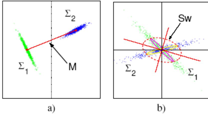
Fig. 1. a) Two normal distributions with different orientations and eccentricity ratio. b)  $S_w$  geometrical interpretation. The axes of the ellipses has been drawn with standard deviation length.
