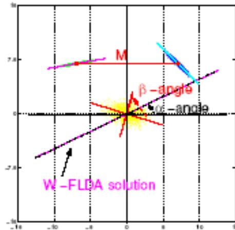
Fig. 3. Distributions and angles: The system is rotated to make the line that passes through the mean points parallel to the x-axis, the yellow ellipse represents  $S_w$ ,  $\beta$  is the angle of the minor axis of  $S_w$  and  $\alpha$  is the angle of  $w$ .
