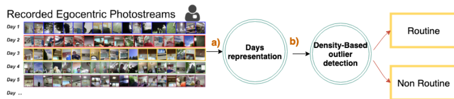
Fig. 2: The pipeline of the proposed model. Given a set of recorded days, a) they are translated to a set of global or semantic features. Later, b) days are considered as routine or non-routine based on their resemblance.
