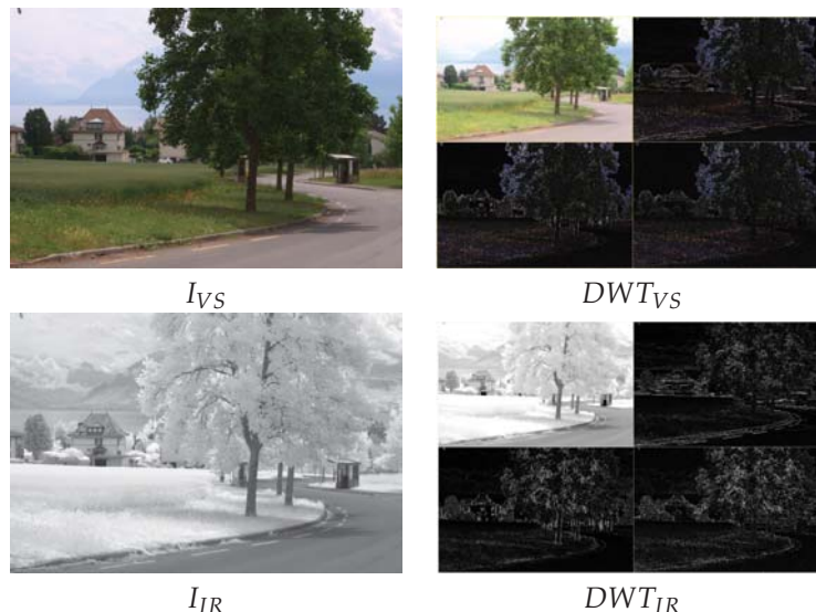
Figure 1. (Left) Pair of images (VS-IR) to be fused; (Right) DWT decompositions (one level) of the input images.
