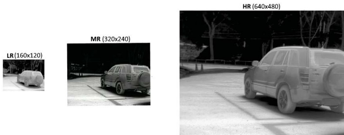
Figure 1: Example of thermal images acquired by each camera. ( left ) LR image with 160x120 native resolution from Axis Domo P1290. ( middle ) MR image with 320x240 native resolution from Axis Q2901-E. ( right ) HR image with 640x480 resolution from FC-6320 FLIR (native resolution 640x512).
