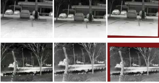
Figure 4: Image registration results. ( top ) From left to right: LR image; MR image; and image resulting from the registration of MR image with the results of SR_{LR} image. ( bottom ) From left to right: MR image; HR image; and image resulting from the registration of HR image with the results of SR_{MR} image.
