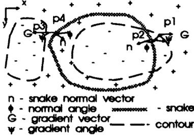
Figure 3: Two examples of pairs of edge points and snaxels with suitable directions ( $p_1, p_2$ ) and with non-suitable directions ( $p_3, p_4$ )
