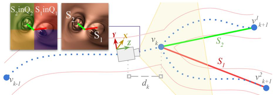
**Fig. 2.** Edge Labelling Procedure: the camera captures an image at distance  $d_k$  from the  $v_k$ , projecting lines to children at level  $k + 1$ . Image is split into quadrants to label line segments  $S_1$ ,  $S_2$ .
