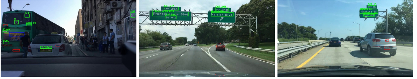
Fig. 3: Example frames from clips in RoadText-1K with text location and transcription annotations overlaid. Boxes in green correspond to English text, blue represent non English and red represent illegible text.
