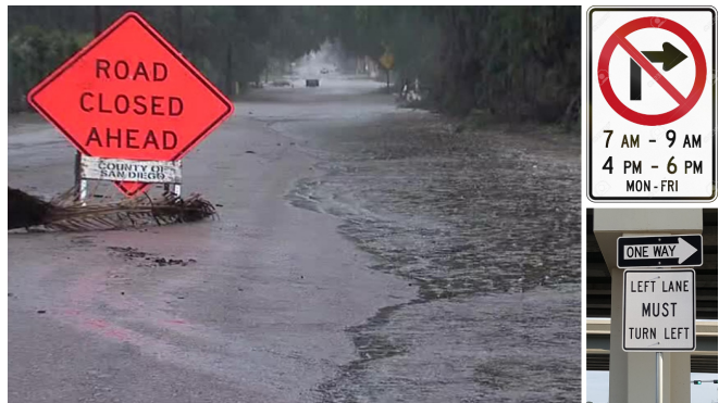
Fig. 1: Examples showing the importance of text for self-driving and advanced driver assistance systems. Navigation systems in the case of scene on the left, without cognizance of text would be taking the road while it is not supposed to. Similarly the scene at the top-right shows no right turn, but the restriction is only for the timings mentioned. The image on the bottom-right has one way sign to the right but has conflicting message through text.
