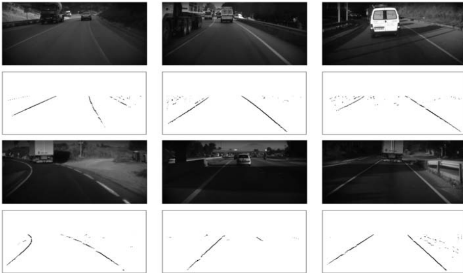
Figure 7 Detection under challenging conditions. From left to right, top to bottom, original and ridge images corresponding to: worn off paint, tire marks, white vehicle, high curvature, inside a tunnel, cast shadows
