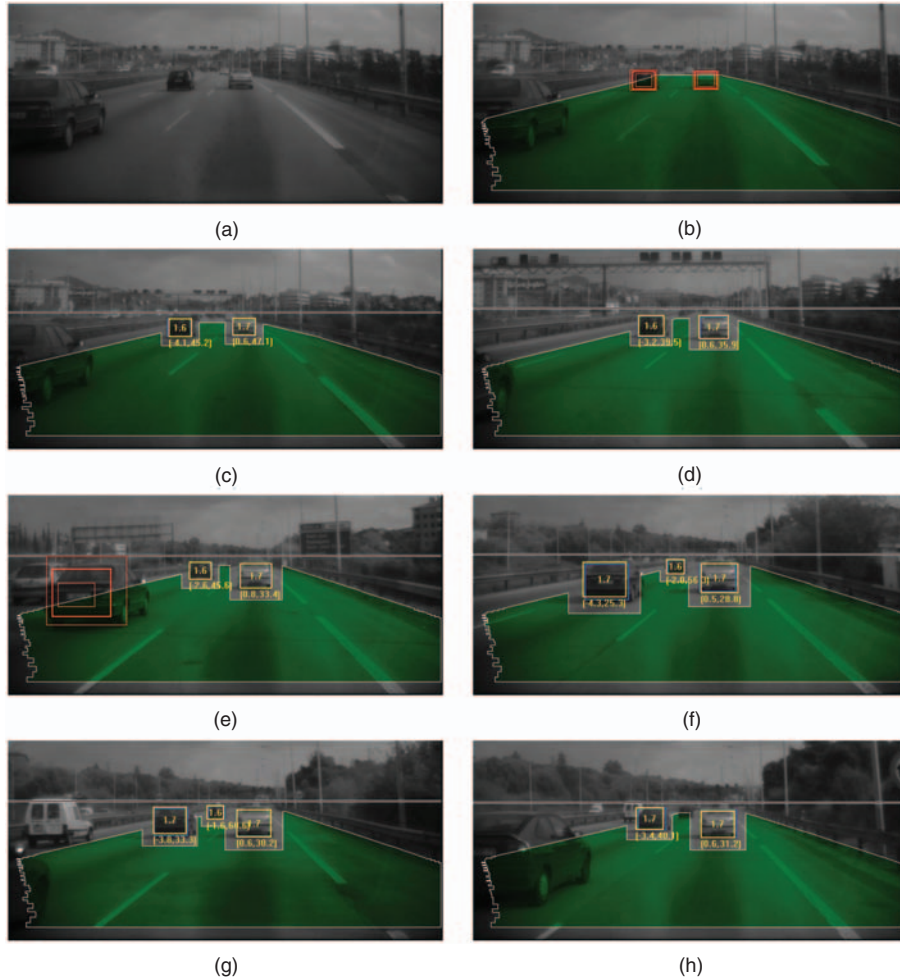
Figure 12 Example of the system performance. (a) First frame of the sequence. After several consecutive detections (b) new targets are added to the tracking module (c). This is represented by a yellow rectangle outlining the vehicle, where the estimation of its width and road location is numerically indicated. These targets are properly tracked in the following frames (d). New vehicles entering in the scene are properly detected (e) and tracked (f). Vehicles outside the inspection region are ignored (g). At far distances, very occasionally mistracking events occur (h)
