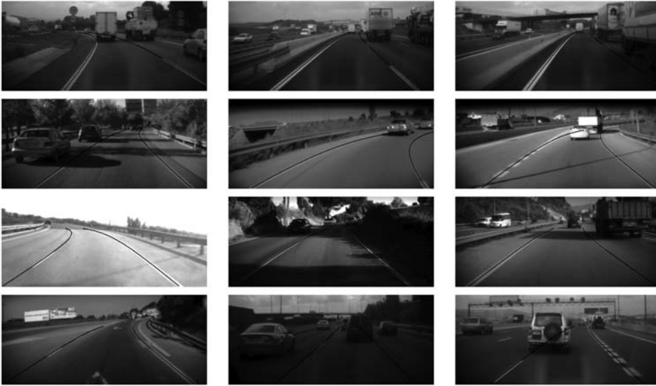
Figure 9 Segmented lane curves on frames acquired by different cameras: dashed lines, occlusion, special road marks, shadows
