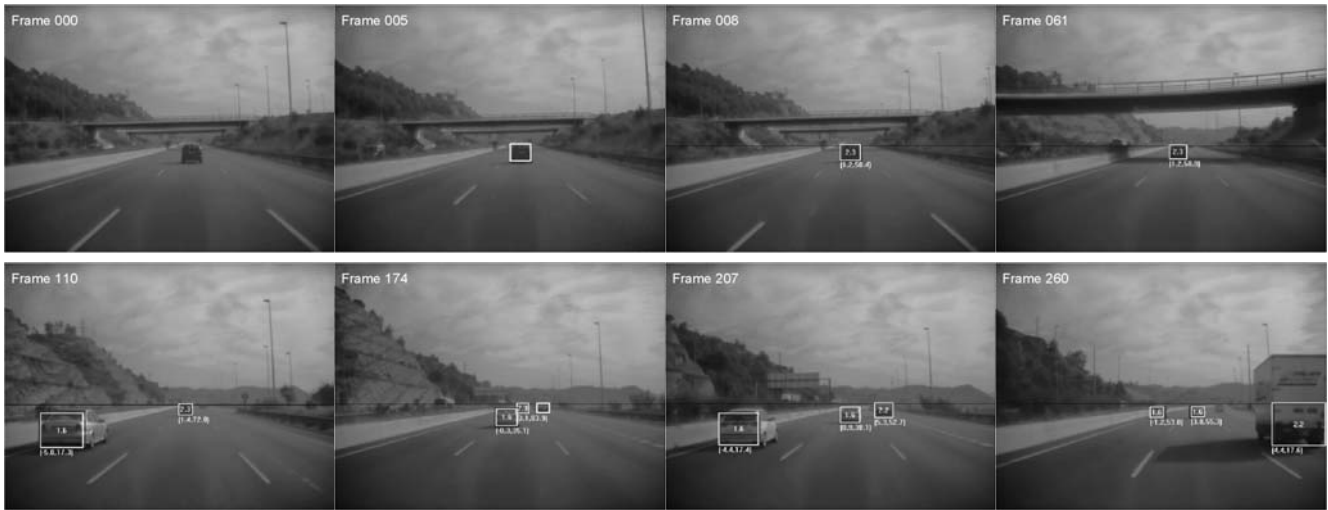
Fig. 9. Detection-tracking procedure. Frame 000 is the first frame of the sequence. After several consecutive detections (frame 005), a target is added to the tracking module (frame 008). Frame 061 shows that the tracker is robust to sudden changes in the lightening conditions. At frame 110 a new target is added to the tracking module. Frame 174 shows the situation previous to the elimination of one target, due to the occlusion it suffers. Also it is shown how a distant truck is detected. Frame 207 show the simultaneous tracking of two cars and one truck. Frame 260 shows the situation previous to the elimination of one target that leaves the camera field of view.
