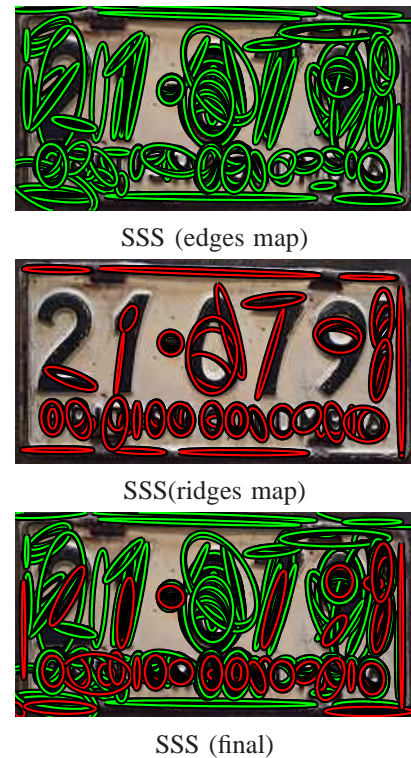
Fig. 5. An example of the proposed region pruning. The detected regions are replaced by fitted ellipses.
