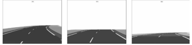
Figure 13. A negative slope change shrinks the road region from the image, causing large errors in the computed parameters.
