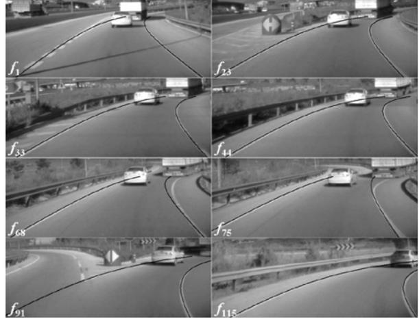
Figure 7. Several frames of a sequence at 10 fps. The vehicle leaves a highway, finds a bifurcation and turns to the right. Notice that in spite of the high curvature of the lane lines the method is able to detect them very well, except in the frames where the two lines are not parallel ( $f_{68}$  and  $f_{75}$ ) due to the approaching bifurcation.
