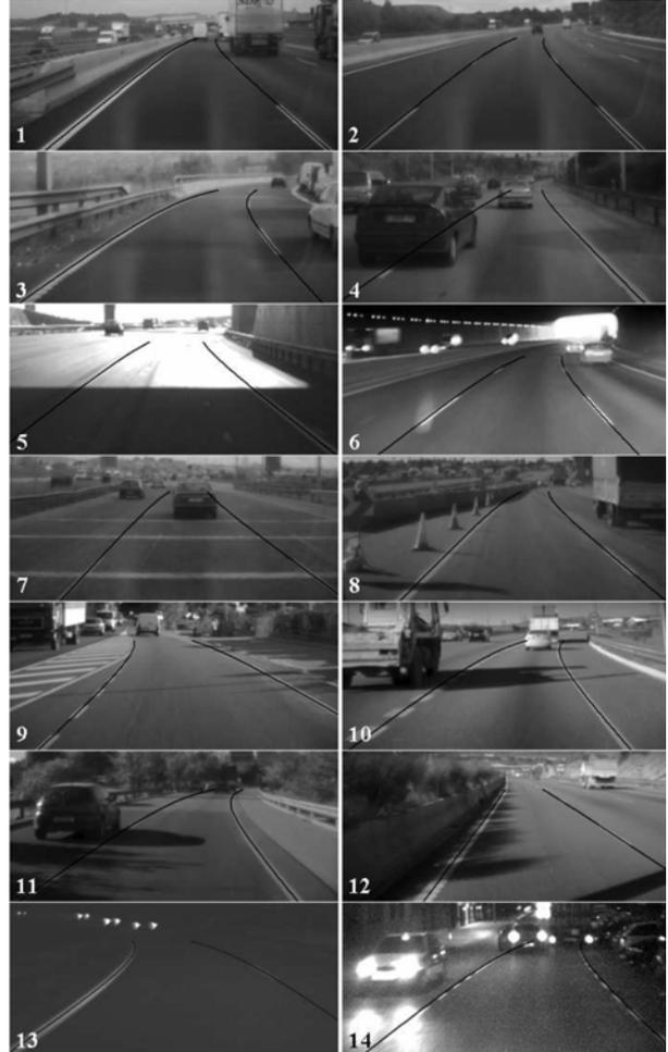
Figure 9. Segmented lane curves on frames acquired by different cameras: (1-3) dashed lines, (4) occlusion. (5,6) tunnel exit and entrance, (7) horizontal marks, (8) cones, (9,10) special road marks, (11,12) shadows, (13,14) night images with low contrast and reflections.
