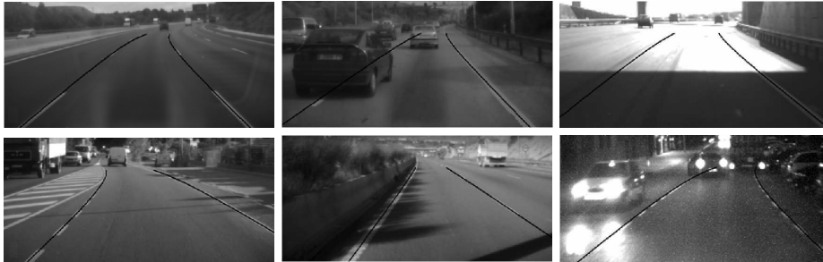
Fig. 3. Segmented lane line curves. From left to right and top to bottom : dashed lines, occlusion, tunnel exit, special road marks, shadows, night image with reflections. Complete sequences from which these frames have been extracted can be viewed at www.cvc.uab.es/adas/projects/lanemarkings/IbPRIA07.html .
