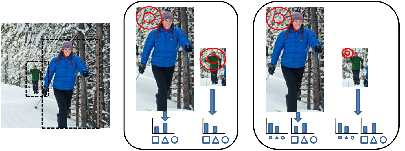
Fig. 2. Scale coding: (left) input image, superimposed bounding boxes indicate persons performing an action; (middle) in standard scale coding the scale is independent of the object size (red circles show the extracted feature scales), and they are all assembled in a single histogram per image; (right) our proposal of relative scale coding adapts to the bounding box of the object. This ensures that similar structures (such as hands and ski poles) are captured at the same scale independent of the bounding box size. The features are represented in several concatenated histograms which collect a range of feature scales.
