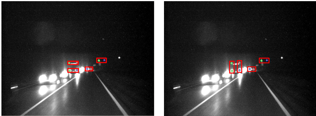
Figure 6: Sequence 2: one bus approaching the camera (four feature points), one car in the same direction as the camera and two lamp posts. Left: Costeira–Kanade method. Right: Han–Kanade method. In both methods the features of the bus are not grouped as a unique object, due to the perspective effect (in the last frames the bus is very close to the camera).
