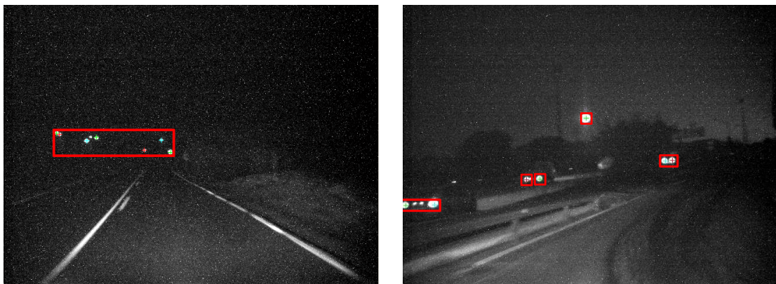
Figure 7: Left: Costeira–Kanade method. Sequence 4: seven static points, segmented as one object. Right: Han–Kanade method. Sequence 14: three cars in the same direction as the camera and one lamp post. The features of the second car are segmented separately.
