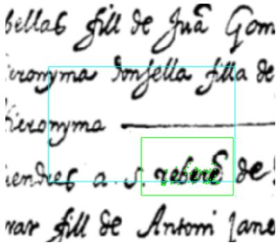
Fig. 2. The searched word in the sliding window is found and the extent of the word, depicted as a green box, which is computed using the matching key points, depicted as green dots.
