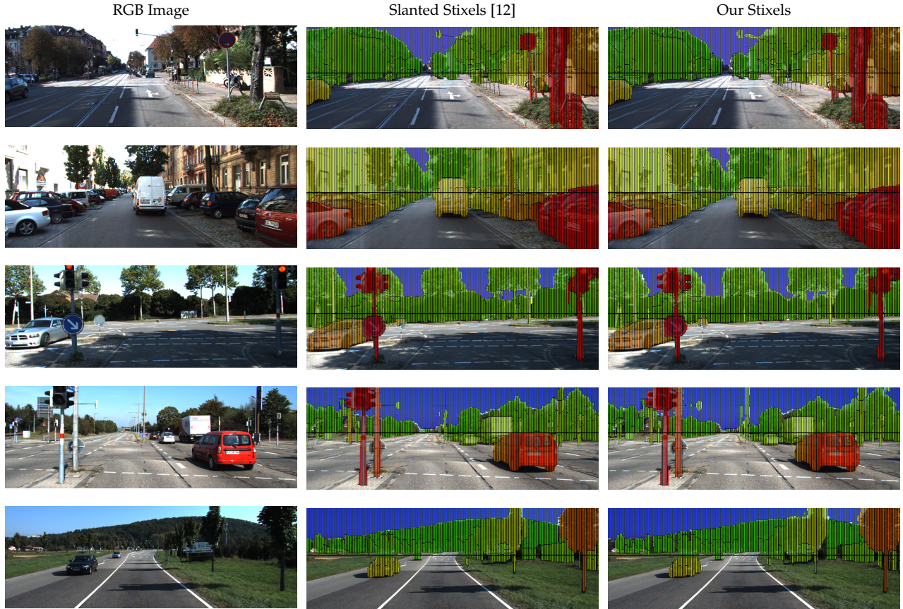
Fig. 6: Exemplary outputs on real data (KITTI 15): RGB Image (left), Slanted Stixels [12] (center) and Our Stixels (right) representations are shown. Color encodes the distance from close (red) to far (green). As we can see, the representation of our proposal is visually similar to the baseline.
