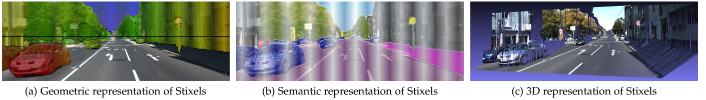
Fig. 1: Scene representation of a challenging street environment obtained by our method. Geometric or Depth (left), semantic (center) and 3D (right) representations are shown. In fig. 1a, color encodes depth from close (red) to far (green). In fig. 1b, color encodes the semantic class following [21].
