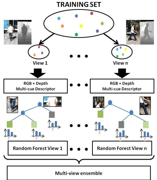
Fig. 2. Multi-view, Multi-cue, Multi-modal detector scheme. 1) Split training set samples in different views. 2) Generate a multi-modal representation using RGB and depth. 3) Extract multi-cue features. 4) Train a random forest of local experts for each view. 5) Ensemble different views detection.
