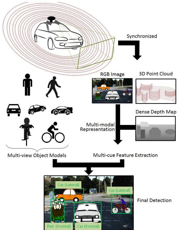
Fig. 1. General scheme: From RGB images and LIDAR data to object detection. RGB images and LIDAR data synchronized for multi-modal representation. Multi-modal representation based on RGB images and dense depth maps (obtained from LIDAR sparse data). Multi-cue feature extraction over the multi-modal representation. Multi-view detection of different objects.
