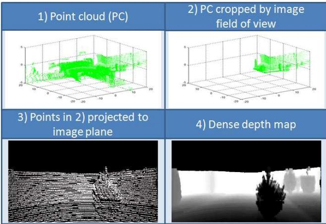
Fig. 3. Dense depth map generation scheme. From a cloud of points to a dense depth map: Filter cloud of points for synchronize with view field of image. Projection of 3D points into 2D image coordinates. Interpolate depths for getting a dense depth map.
