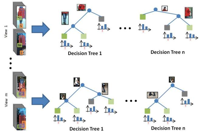
Fig. 4. Multi-View Random Forest scheme. For each view is learnt a different random forest, and each tree has different configuration of random patches.
