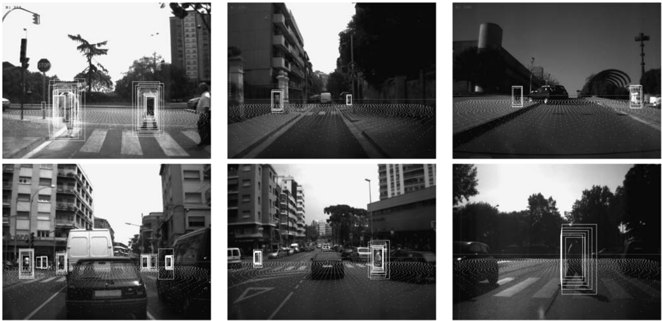
Figure 6. Pedestrian detection . Some examples showing detected pedestrians, including false positives not corresponding to our target. (Raw detection without any kind of post-processing, fixing the grid using the estimated pitch).
