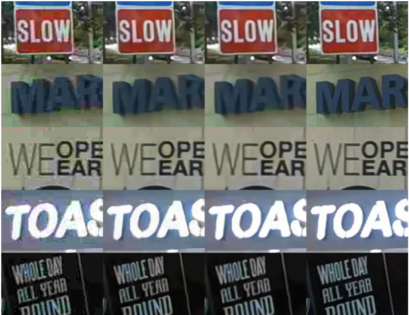
Figure 6: Examples of cropped text reconstruction. The leftmost column shows compressed versions of cropped text at QF 10, the second column is the reconstruction using the whole image sampling strategy, the third shows the reconstruction using the cropped text sampling strategy and the rightmost column is the ground truth.
