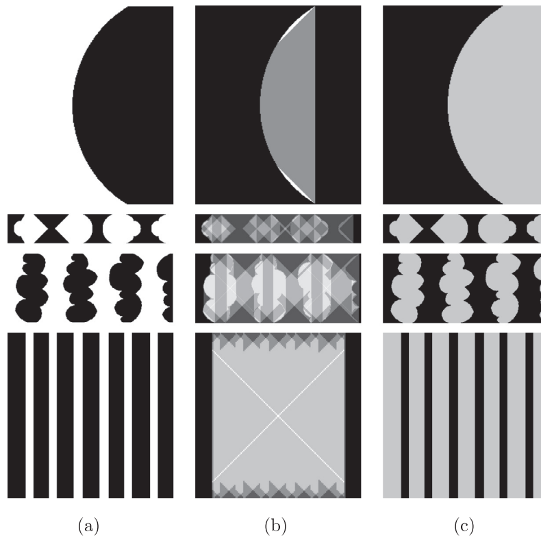
Fig. 4. Modeling convexity: (a) original image. (b) Image whose intensity values correspond to the beliefs computed through multi-directional linear voting taking into account only convexity. Pixels with high intensity values have a high belief to be part of a foreground region. (c) Normalized probability of foreground after averaging on homogeneous regions.
