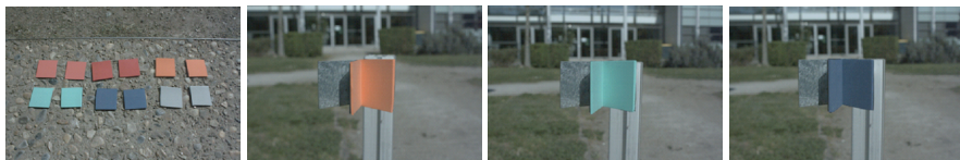
Figure 5: Images of the patches used for the real experiments. Left image: the six patches acquired as planar surfaces, without inter-reflections (2 samples per patch). The three right images: three of the six patches acquired as folded surfaces.
