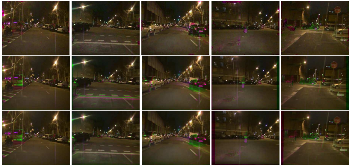
Figure 5: Alignment instances in negative color for (first row) SIFT-flow, (second row) GDB-ICP and (third row) ECC algorithm based on the frame pairs between the top and bottom row in Fig. 4.
