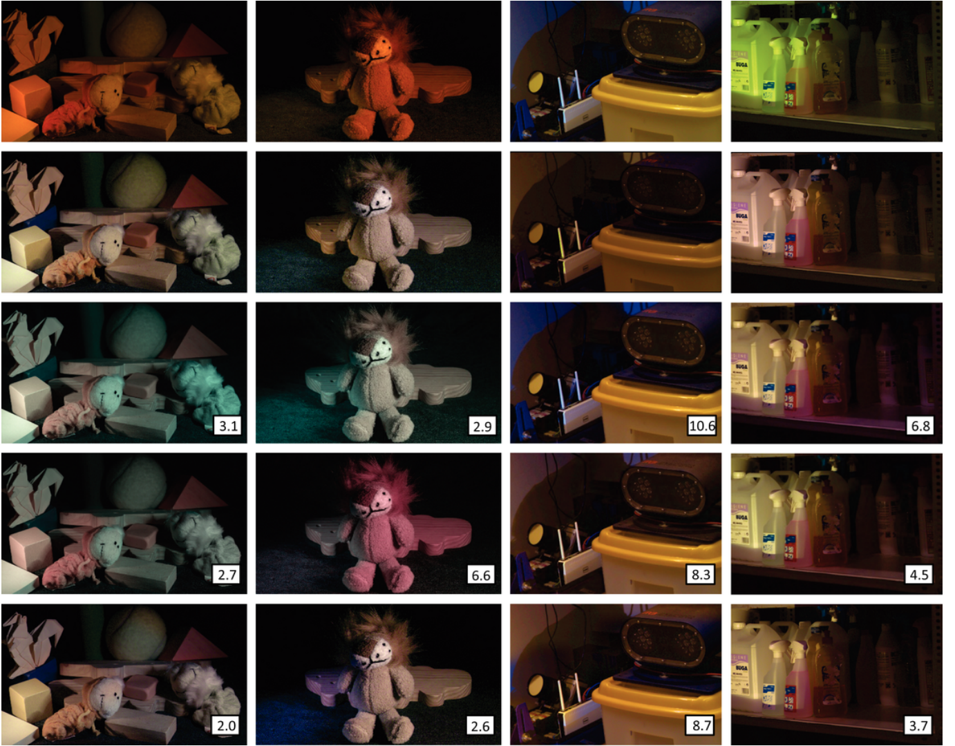
Fig. 4: Examples of automatic white balance (WB). From top to bottom the rows present: original images, the corresponding WB images using the ground truth, global grey world, Gijsenij et al. [23], and MIRF accordingly. Note that the images have been converted to sRGB for better visualization. The captions of each image denote the mean angular error in the WB image.
