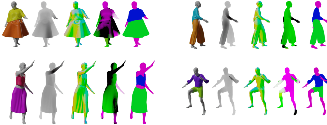
Figure 14: CLOTH3D data representations. From left to right: RGB, depth, normals, velocities, and segmentation masks.
