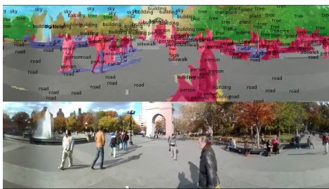
Fig. 9. Example of the result obtained (top) by applying a scene parsing algorithm to a conventional non-egocentric image (bottom). We can see the different segments found (separated by different colours) and the classes assigned to each of them. Picture adapted from [33].
