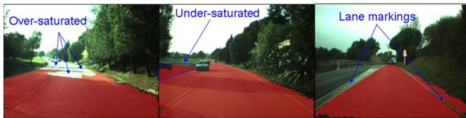
Fig. 13. Examples where our road-detection method currently fails.
