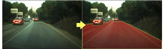
Fig. 1. Aim of vision-based road detection is identifying road pixels in an image.
