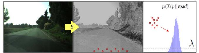
Fig. 7. (Left) Color image  $I_{RGB}$ . (Middle) Corresponding  $\mathcal{I}$  computed using the invariant angle  $\theta$ . (Right) Nonparametric road model built using the normalized histogram formed with the surrounding region of several seeds (nine in this case) placed at the bottom part of  $\mathcal{I}$ .
